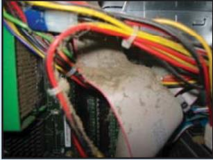
*Photograph of an actual client's computer. Notice the lint accumulated on the CPU cooling assembly. This machine was suffering from random reboots. After our professional cleaning service, the client reported no more problems!*
