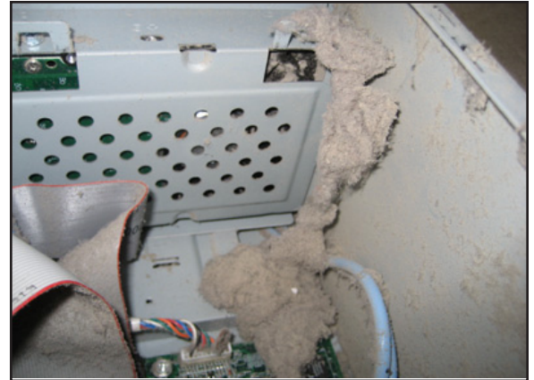
When this computer came into our shop, the client was complaining of slow performance, random lockups and the computer shutting down without any kind of warning. When we opened the case, we found out why - layer upon layer of lint and dust had caked up on the cooling fans, causing the computer to overheat.
